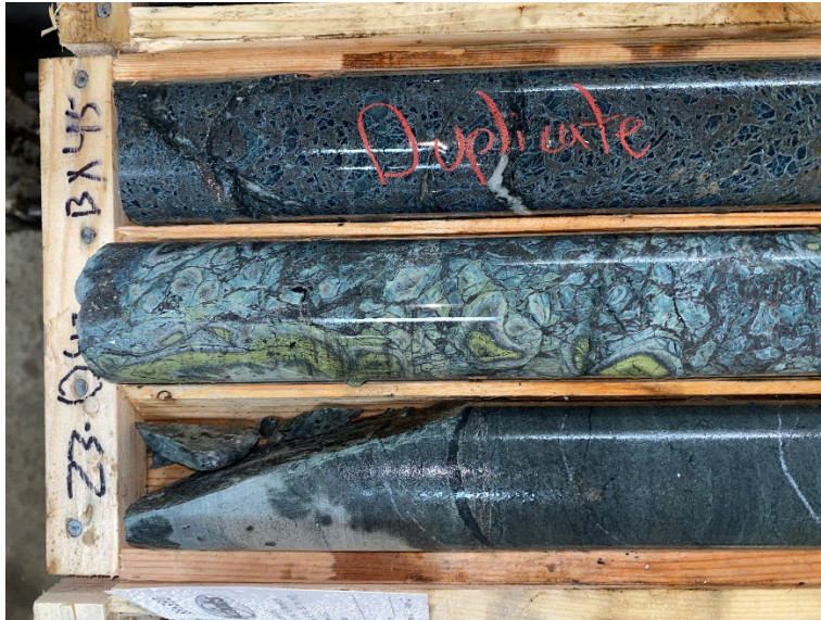
Figure 2 Blue breccia with unknown blue mineral and green epidote clasts (second row), at 194.5 m, sample 889876, PG-23-1.
