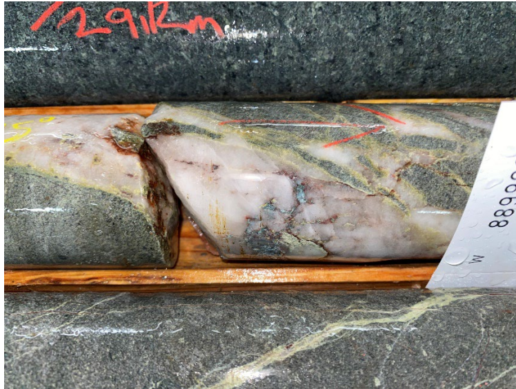
Figure 4 Quartz vein with epidote-sericite-chlorite-hematite at 30.32 m, sample 889907, PG-23-2.
