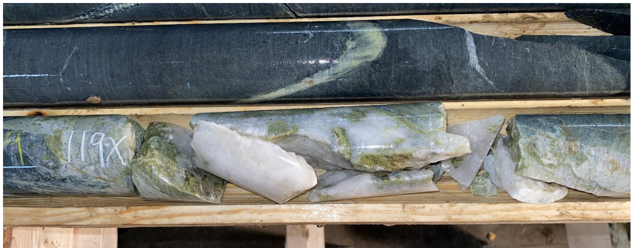
Figure 3 Quartz vein with green epidote, yellow-brown ankerite and small dark red garnets at 119 m, PG-23-1.
