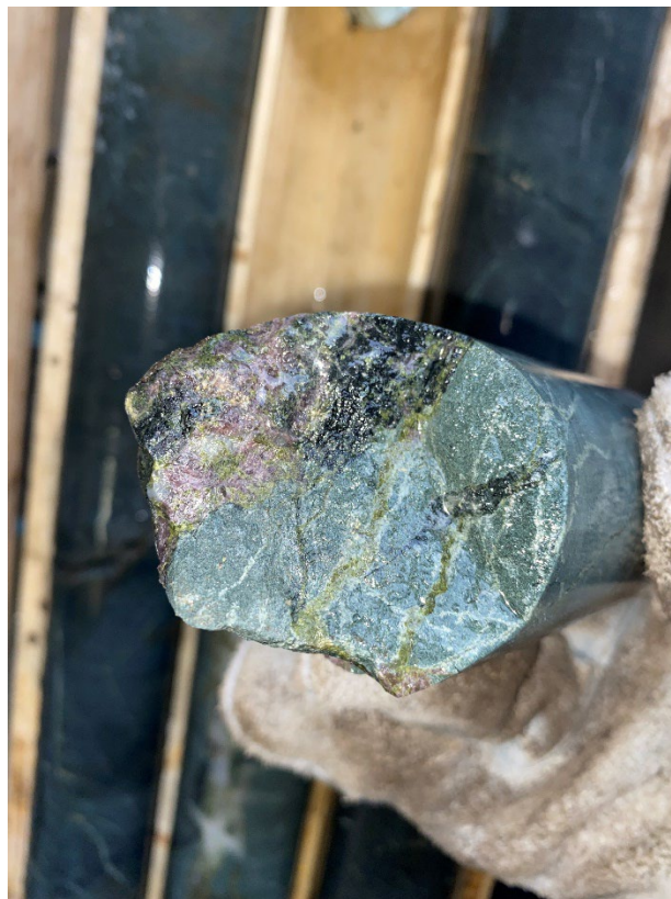
Figure 5 Secondary purple fluorite with green epidote and sulphides at 135m, sample 889925, PG-23-2.
