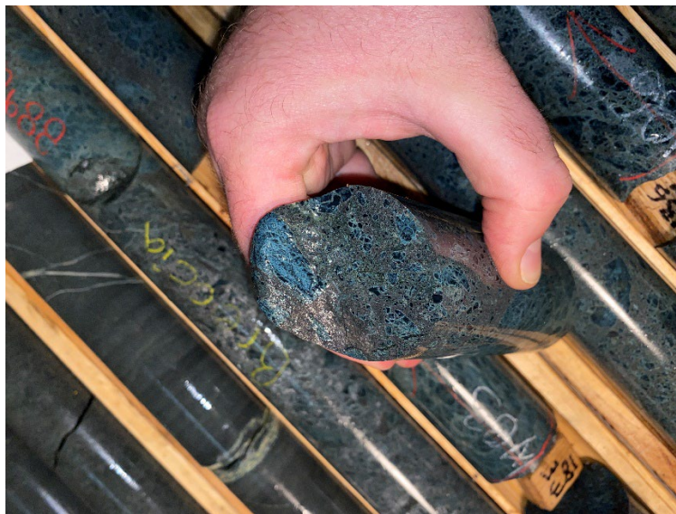
Figure 1 Blue breccia with up to 35% sulphides in the matrix, at 183 m, sample 889863, PG-23-1.
